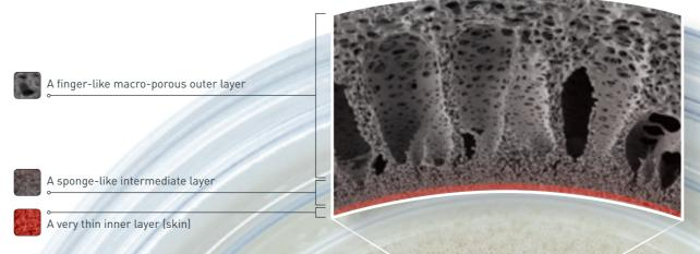
THE **THERANOVA** DIALYZER EFFECTIVELY TARGETS MIDDLE MOLECULES, IN AN EQUIVALENT WAY TO HDF IN HIGH CONVECTIVE VOLUME MODE  $^{10}$
